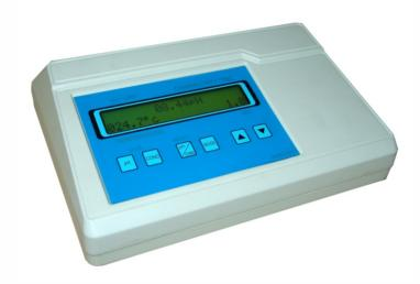
PH/ ORP/Conductivity/TDS meter is a unique test tool to measure the pH, Conductivity, Total Dissolved Solids, ORP values of various solutions and chemicals. Used in various educational institutes, research laboratories this instrument measures the pH, Conductivity, ORP, TDS, salinity mode, resistivity mode, °C mode with accuracy.
